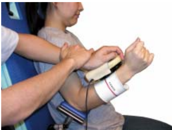
Figure 3: Measurement of elbow flexion torque (source: http://www.nite.go.jp/ )
